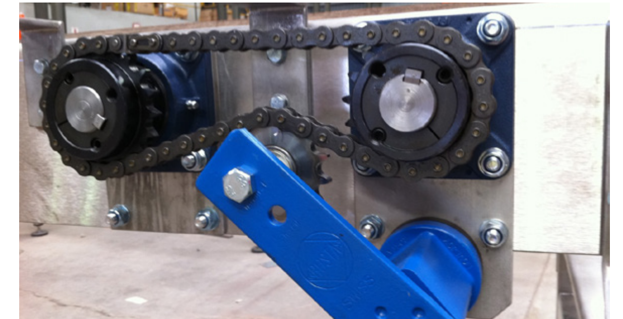
Tensioner on food packaging machine designed with ROSTA SE ®
