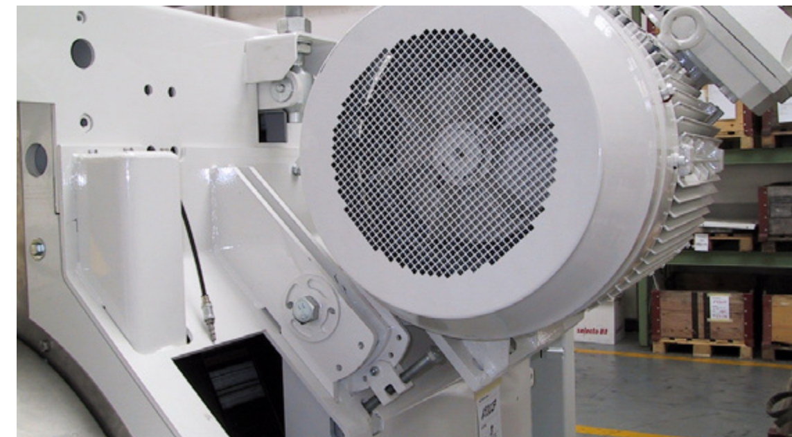
MB on milling machine designed with ROSTA MB ®
