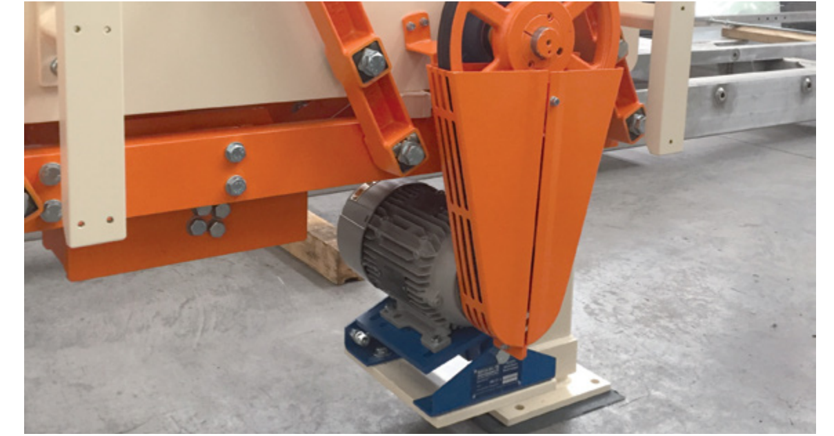
Tobacco Conveyor designed with ROSTA MB ®
