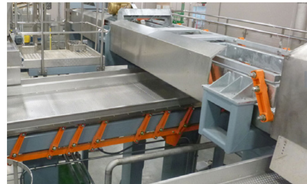
Tobacco conveyor designed with customized ROSTA AD ®
