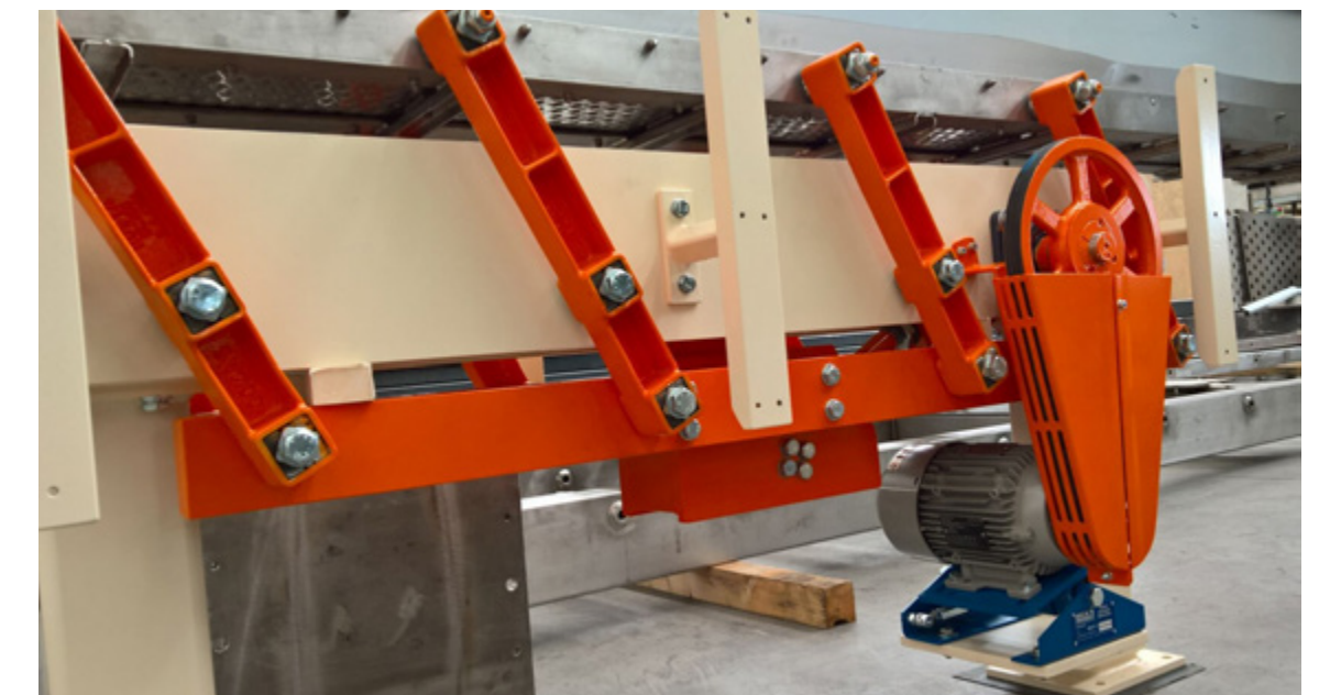
Tobacco primary feeder with customised ROSTA AD ®
