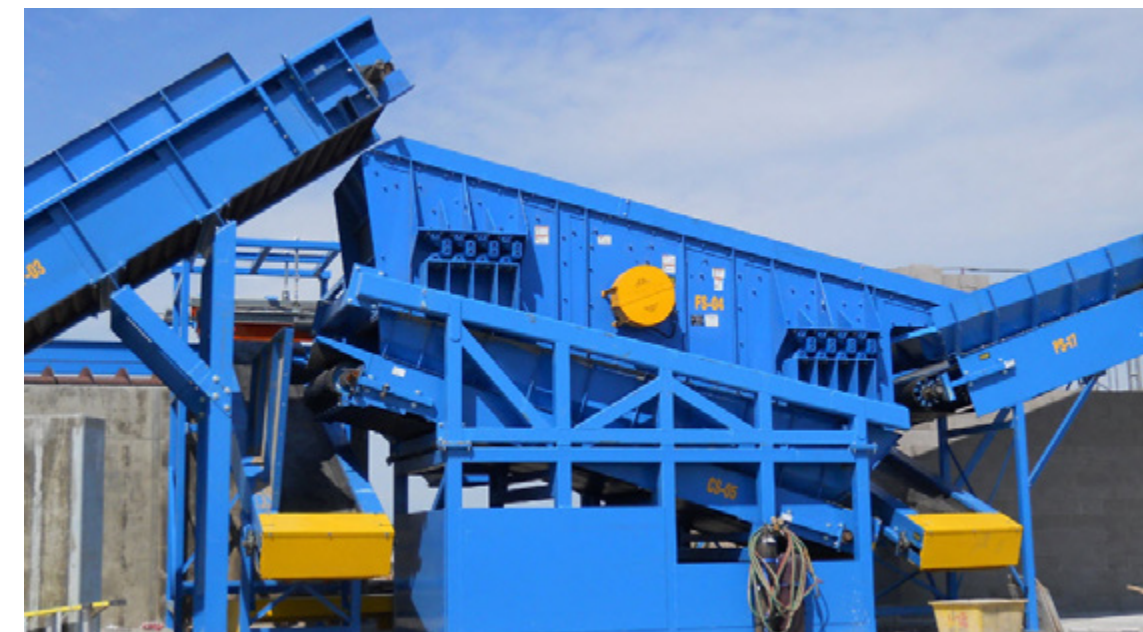
Fixed plant vibrating screen suspension designed with ROSTA AB ®
