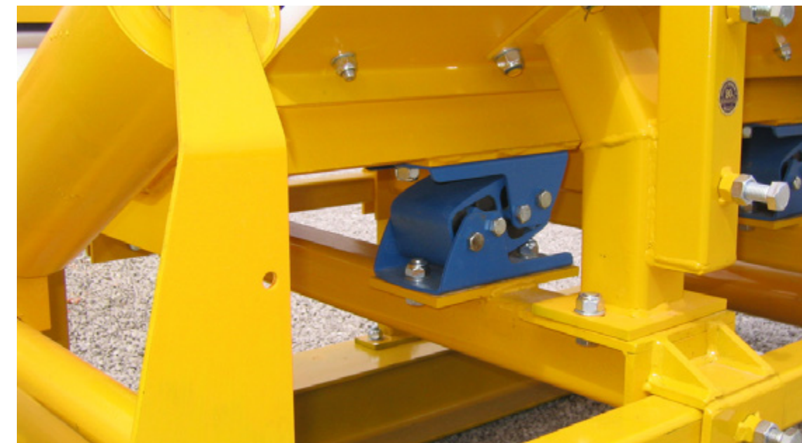
Conveyor impact table designed with ROSTA ESL ®
