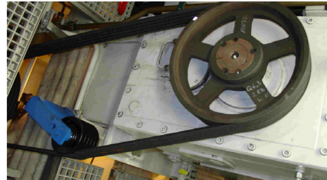
Conveyor gearbox drive designed with ROSTA SE ®
