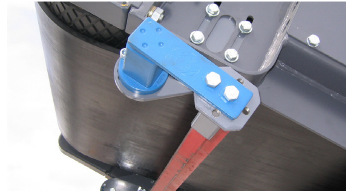
Belt scraper designed with ROSTA SE ®
