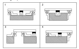
Pillow blocks shown are the standard SSUPB0 or SPB-OPN style. To order System 1DA with standard pillow blocks, order the Side Mounted Shaft Rail Assembly (SSRA) and the SSUPB0 or SPB-OPN separately.
