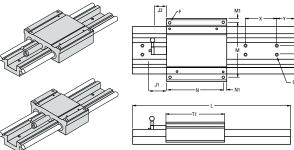
Dual Shaft Rail Supported Cross-Section
