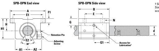
† Size .500 has oil lubricant fitting. Sizes .625 and above have 1/4-28 access for lubrication.
