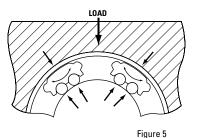
Super Smart Ball Bushing Bearing Self-Alignment
