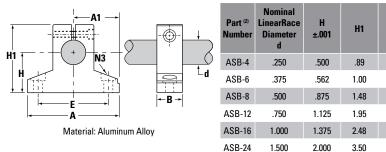
Type SB 60 Case LinearRace Shaft End Support Blocks (Dimensions in inches)
