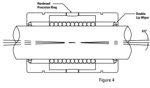
Super Smart Ball Bushing Bearing Self-Alignment Feature
