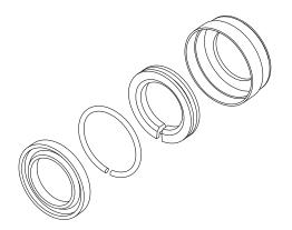
Lube for Life modification kits provide continuous bearing lubrication and enhanced protection for a broad range of applications. The Lube for Life attachments consist of a section of oil saturated polymer actively compressed by a contact spring, inside a standard Pillow Block seal. Mod Kits are for use with non self-lubricating Super and Super Smart Ball Bushing bearing Pillow Blocks. Each Mod Kit includes 2 Lube-for-Life cartridges and assembly instructions.
