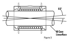
Super Ball Bushing Bearing Self-Alignment Feature
