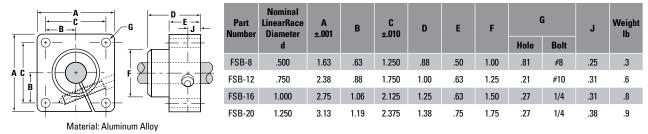
Type FSB Flanged 60 Case LinearRace Shaft End Support Blocks (Dimensions in inches)
