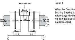
When the Precision Steel Ball Bushing Bearing is installed in its standard Pillow Block it will self-align up to 3 degrees
