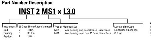
60 Case LinearRace Specifications Material: 440 Stainless Steel Hardness: 55 HRC minumum Surface Finish: 4 R<sub>a</sub> microinch Straightness: .0001 inch per inch
