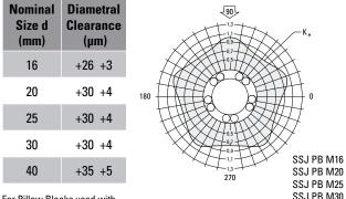
For Pillow Blocks used with LinearRace Shaft, h6 tolerance
