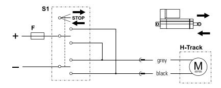
To extend the actuator, apply +Vdc to black -Vdc to grey. To retract, apply -Vdc to black and +Vdc to grey. Avoid running the actuator in to the ends.
